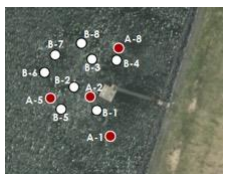
Utility 2 Disk Aeration System
