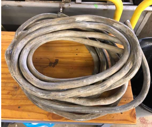
Typical ~ 3/4 inch lead service line removed from ground, coiled (material is flexible!)
